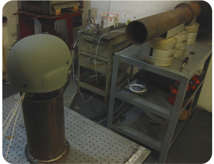
Fig. 5 — Shock tube and advanced combat helmet (ACH) at Purdue University Zucrow’s Laboratory. The pressures measured during the physical tests were compared to simulation results to benchmark the FEA models.
