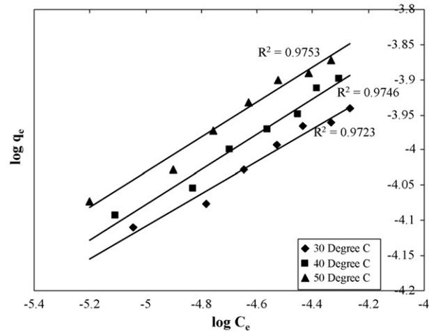
Fig. 3. Freundlich adsorption isotherm for Tartrazine–hen feather system: temperature = 50 °C; pH 2.0; amount = 0.01 g; time = 24 h.
